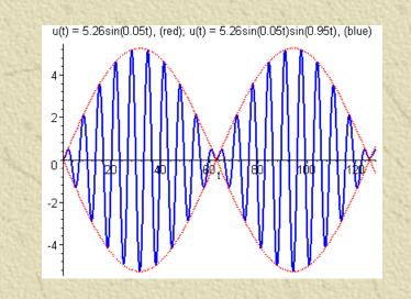
Undamped Equation: General Solution for the Case  $\omega_0 = \omega$  (1 of 2) \* Recall our equation for the undamped case:
