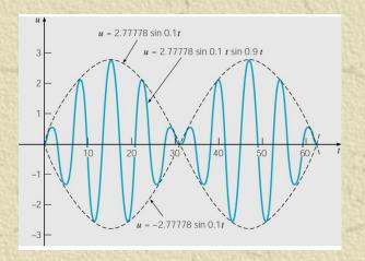
Example 3: Undamped Equation, Mass Initially at Rest (1 of 2) Consider the initial value problem  $u''(t) + u(t) = 0.5 \cos 0.8t$ , u(0) = 0, u'(0) = 0Then  $\omega_0 = 1$ ,  $\omega = 0.8$ , and  $F_0 = 0.5$ , and hence the solution is  $u(t) = 2.77778 (\sin 0.1t) (\sin 0.9t)$
